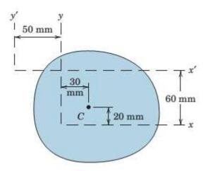
Problem 4. Determine the product of inertia of the shaded area about the x-y axes.
