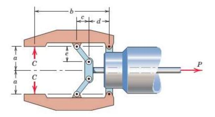
**Problem 2.** Determine the force F between the jaws of the clamp in terms of a torque M exerted on the handle of the adjusting screw. The screw has a lead (advancement per revolution) L, and friction is to be neglected.
