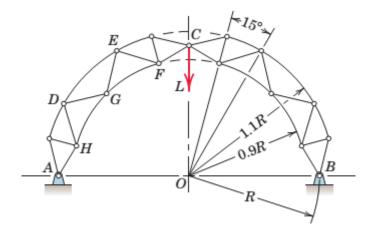
**Problem 8.** In the traveling bridge crane shown all crossed members are slender tie rods incapable of supporting compression. Determine the forces in members DF and EF and find the horizontal reaction on the truss at A. Show that if CF = 0.0, DE =0.0 also.
