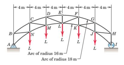
Problem 6. Determine the force in member DG of the loaded truss.
