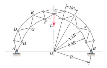
**Problem 8.** In the traveling bridge crane shown all crossed members are slender tie rods incapable of supporting compression. Determine the forces in members DF and EF and find the horizontal reaction on the truss at A. Show that if CF = 0.0, DE =0.0 also.
