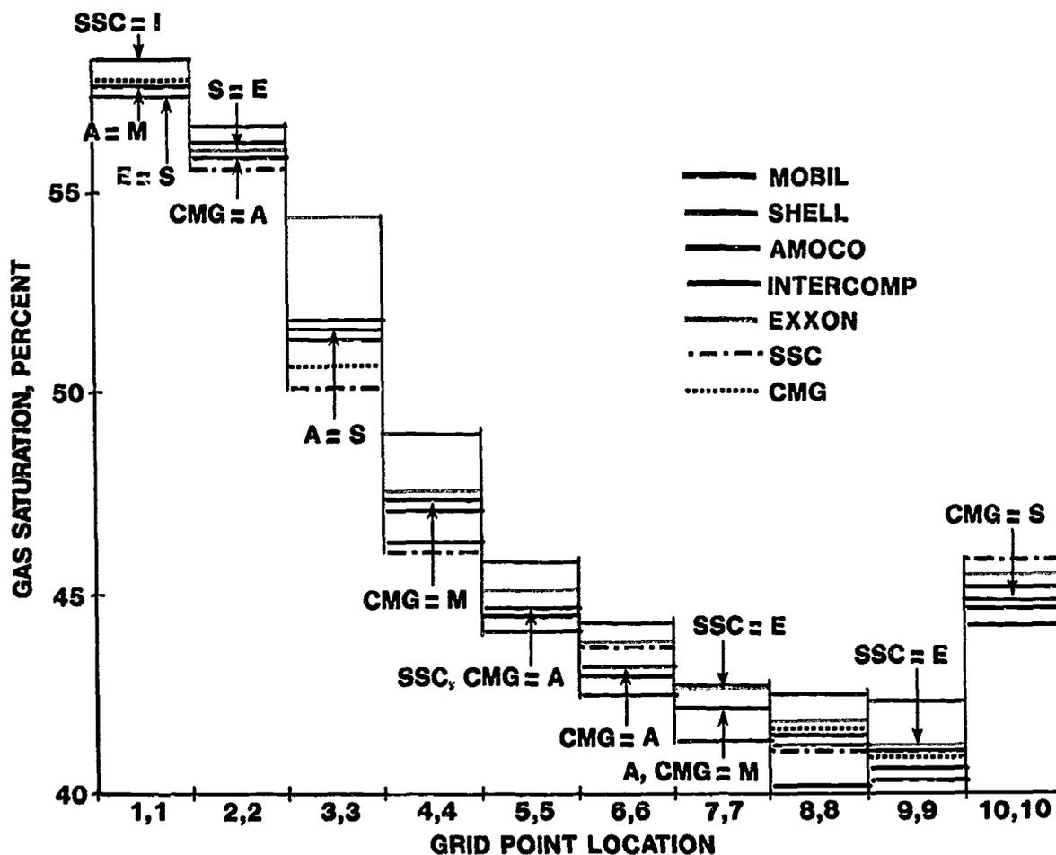
Fig. 17 - Case 2 - gas saturation vs. grid-point location, time = 8 years, top layer.
