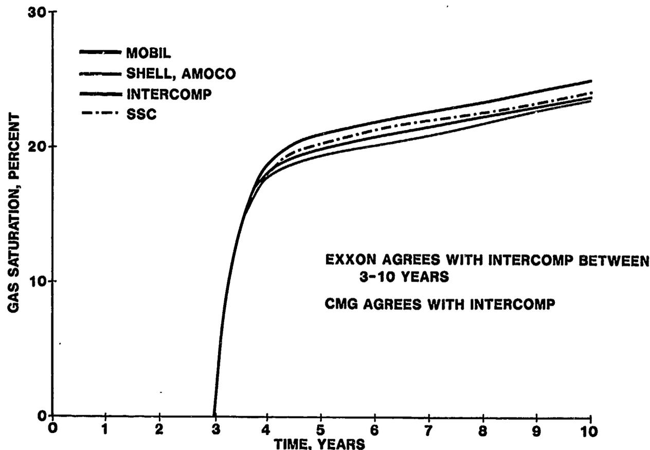
Fig. 14 - Case 2 - gas saturation vs. time for producing well Cell 10, 10, 3.
