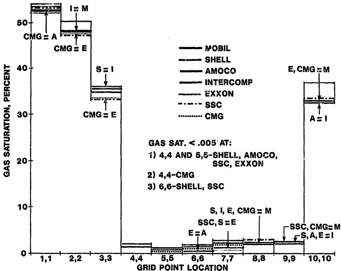
Fig. 18 - Case 2 - gas saturation vs. grid-point location, time = 8 years, middle layer.
