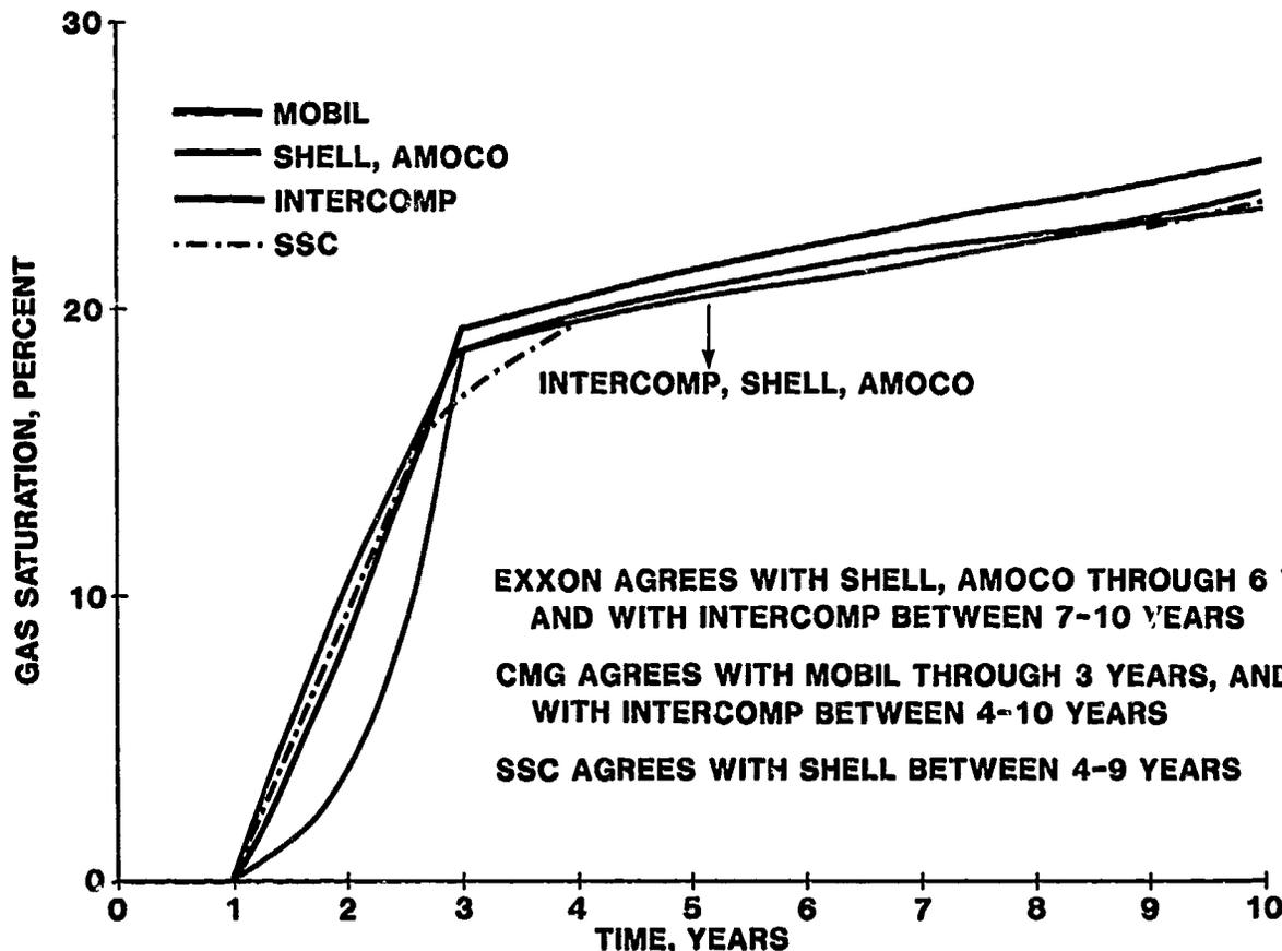
Fig. 6 - Case 1 - gas saturation vs. time for producing well Cell 10, 10, 3.
