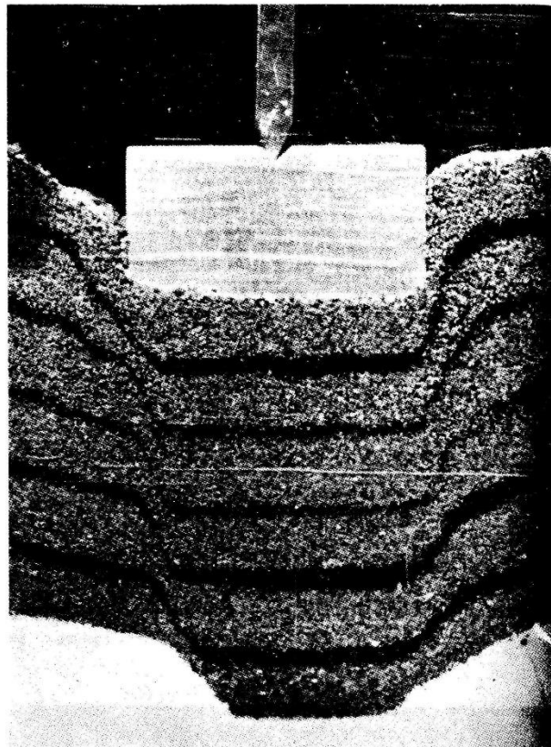
Punching shear failure of a rectangular footing on dense sand underlain by soft clay. (From Vesić, 1970.)
