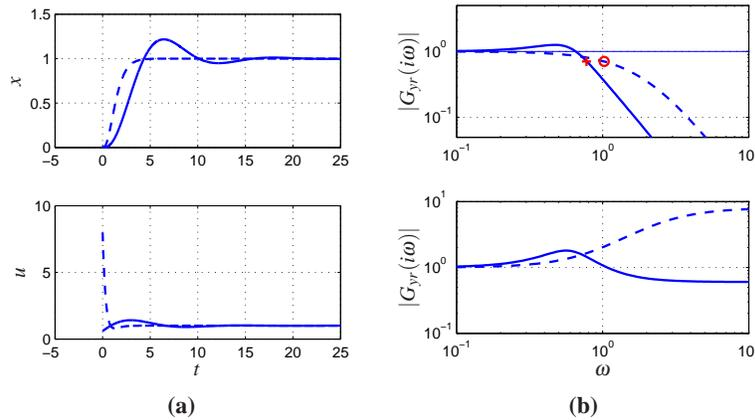
**Figure 11.5:** Reference signal responses. The responses in process output  $y$  and control signal  $u$  to a unit step in the reference signal  $r$  is shown in (a) and the gain curves of  $G_{yr}$  and  $G_{ur}$  are shown in (b). Results with PI control with error feedback are shown in full lines, the dashed lines show results for a controller with a feedforward compensator.
