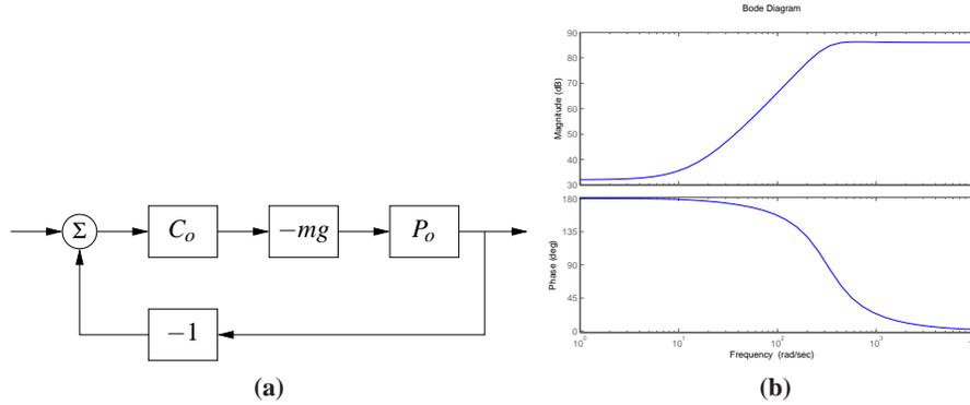
**Figure 11.18:** Outer loop control design for a vectored thrust aircraft. The outer loop approximates the roll dynamics as a state gain  $-mg$ . The Bode plot for the roll dynamics are shown on the right, indicating that this approximation is accurate up to approximately 10 rad/s.
