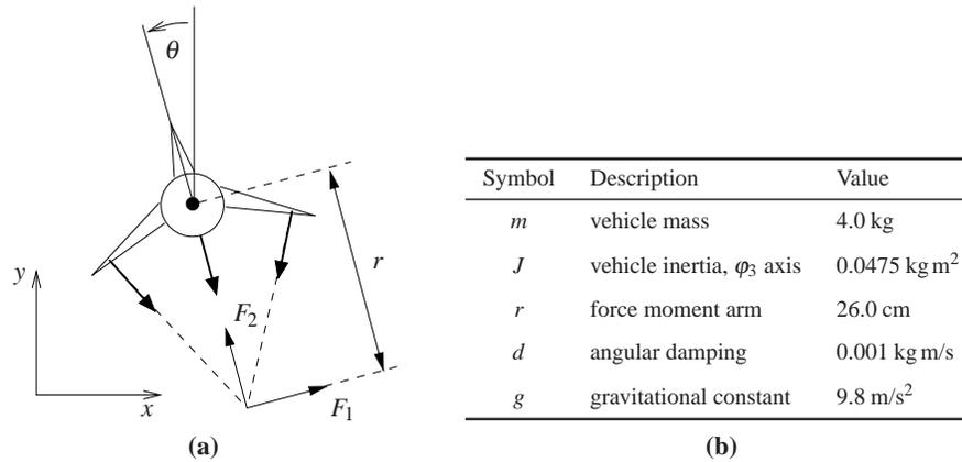
**Figure 11.11:** Roll control of a vectored thrust aircraft. The roll angle  $\theta$  is controlled by applying maneuvering thrusters, resulting in a moment generated by  $F_2$ . The table to the right lists the parameter values for a laboratory version of the system.
