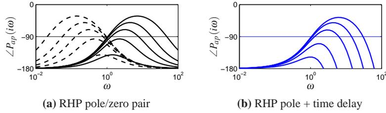
**Figure 11.13:** Example limitations due to the crossover frequency inequality. The figure illustrates limitations by showing the phase of the minimum phase factor  $P_{ap}$  of transfer functions. All systems have a right half plane pole at  $s = 1$ . The system in (a) has zeros at  $s = 2, 5, 10, 20$  and  $50$  (full lines) and at  $s = 0.5, 0.02, 0.1, 0.05$  and  $0.02$  (dashed lines). The system in (b) has time delays  $\tau = 0.05, 0.1, 0.2, 0.5$  and  $1$ .
