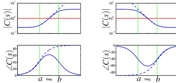
**Figure 11.9:** Frequency response for a lead and lag compensators,  $C(s) = k(s+a)/(s+b)$ . Lead compensation occurs when  $a < b$  (left) and provides phase lead between  $\omega = a$  and  $\omega = b$ . Lag compensation corresponds to  $a > b$  and provides low frequency gain. PI control is a special case of lag compensation and PD control is a special case of lead compensations. Frequency responses are shown in dashed curves.
