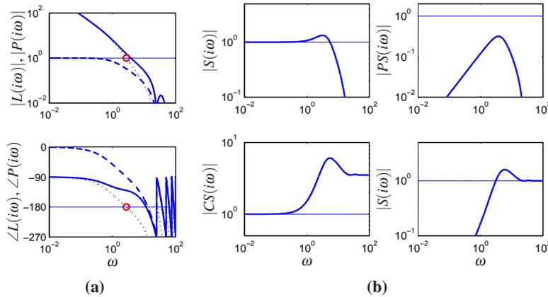
**Figure 11.10:** Loop shaping design of a controller for an atomic force microscope in tapping mode. Figure 11.10a shows Bode plots of the process (dashed), the loop transfer function with an integral controller with critical gain (dotted) and a PI controller adjusted to give reasonable robustness. Figure 11.10b shows the gain curves for the Gang of Four for the system.
