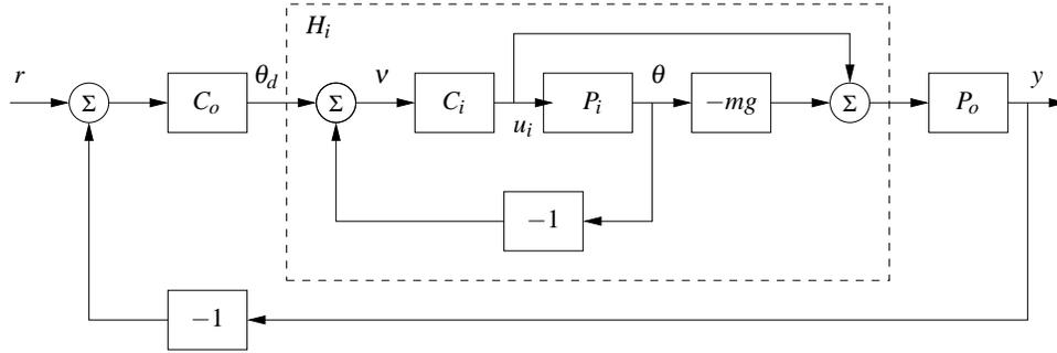
**Figure 11.17:** Inner/outer control design for a vectored thrust aircraft. The inner loop  $H_i$  controls the roll angle of the aircraft using the vectored thrust. The outer loop controller  $C_o$  commands the roll angle to regulate the lateral position. The process dynamics are decomposed into inner loop ( $P_i$ ) and outer loop ( $P_o$ ) dynamics, which combine to form the full dynamics for the aircraft.
