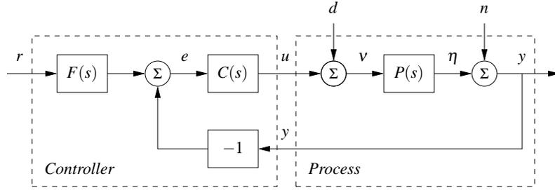
**Figure 11.1:** Block diagram of a basic feedback loop with two degrees of freedom. The controller has a feedback block  $C$  and a feedforward block  $F$ . The external signals are the command signal  $r$ , the load disturbance  $d$  and the measurement noise  $n$ . The process output is  $y$  and the control signal is  $u$ .
