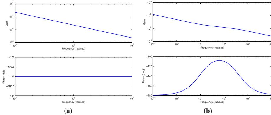
**Figure 11.12:** Control design for a vectored thrust aircraft using lead compensation. The Bode plot for the open loop process  $P$  is shown on the left and the loop transfer function  $L = PC$  using a lead compensator on the right. Note the phase lead in the crossover region near  $\omega = 100$  rad/s.
