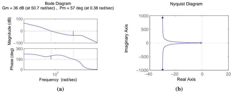
**Figure 11.19:** Inner/outer loop controller for a vectored thrust aircraft. The Bode and Nyquist plots for the transfer function for the combined inner and outer loop transfer functions are shown. The system has a phase margin of  $68^\circ$  and a gain margin of 6.2.
