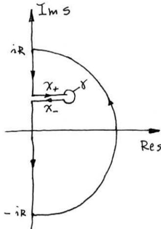
**Figure 11.16:** Contour used to prove Bode's theorem. For each right half plane pole we create a path from the imaginary axis that encircles the pole as shown in the figure. To avoid clutter we have shown only one of the paths that enclose one right half plane.
