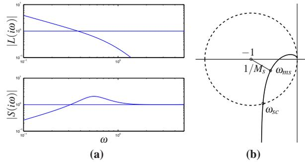
**Figure 11.6:** Graphical interpretation of the sensitivity function. Gain curves of the loop transfer function and the sensitivity function on the right (a) can be used to calculate the properties of the sensitivity function through the relation  $S = 1/(1 + L)$ . The sensitivity crossover frequency  $\omega_{sc}$  and the frequency  $\omega_{ms}$  where the sensitivity has its largest value are indicated in the figure. All points inside the dashed circle have sensitivities greater than 1.
