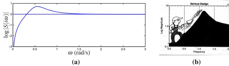
**Figure 11.14:** Interpretation of the *waterbed effect*. The function  $\log |S(i\omega)|$  is plotted versus  $\omega$  in linear scales in (a). According to Bode's integral formula (11.19) the area of  $\log |S(i\omega)|$  above zero must be equal to the area below zero. Gunter Stein's interpretation of design as a trade-off of sensitivities at different frequencies is shown in (b) (from [181]).
