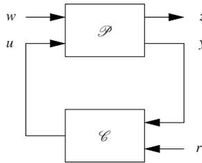
**Figure 11.2:** A more general representation of a feedback system. The process input  $u$  represents the control signal, which can be manipulated, and the process input  $w$  represents other signals that influence the process. The process output  $y$  is the measured variables and  $z$  are other interesting signals of interest.
