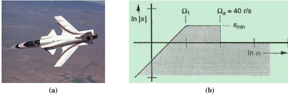
**Figure 11.15:** X-29 flight control system. The aircraft makes use of forward swept wings and a set of canards on the fuselage to achieve high maneuverability. The figure on the right shows the desired sensitivity for the closed loop system. We seek to use our control authority to shape the sensitivity curve so that we have low sensitivity (good performance) up to frequency  $\omega_1$  by creating higher sensitivity up to our actuator bandwidth  $\omega_a$ .
