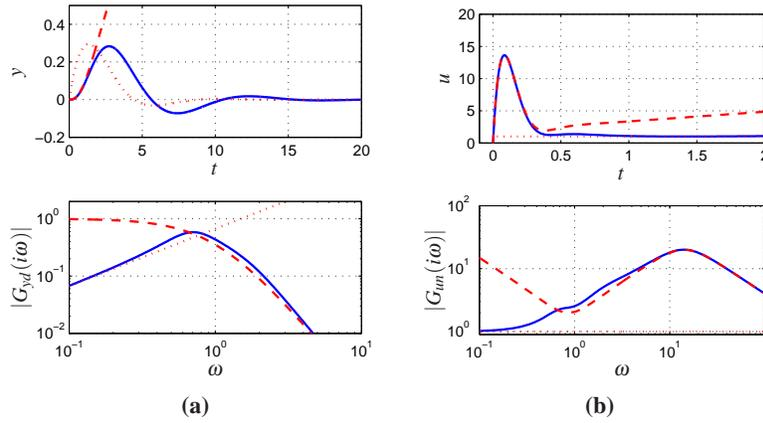
**Figure 11.7:** Disturbance responses. Time and frequency responses of process output  $y$  to load disturbance  $d$  are shown in (a) and responses of the control signal  $u$  to measurement noise  $d$  are shown in (b). The low frequency approximation is shown with dotted lines and the high frequency approximations by dashed lines.
