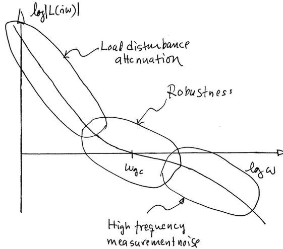
**Figure 11.8:** Gain curve of the Bode plot for a typical loop transfer function. The gain crossover frequency  $\omega_{gc}$  and the slope  $n_{gc}$  of the gain curve at crossover are important parameters that determine the robustness of the closed loop systems. At low frequency, a large magnitude for  $L$  provides good load disturbance rejection and reference tracking, while at high frequency a small loop gain is used to avoid amplifying measurement noise.
