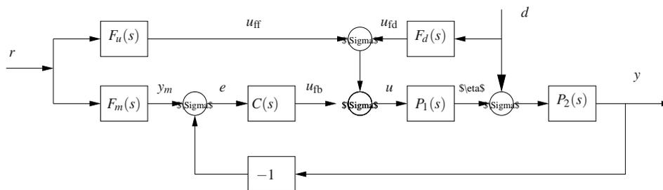
**Figure 11.3:** Block diagram of a system with feedforward compensation for improved response to reference signals and measured disturbances. Three feedforward elements are present:  $F_m(s)$  sets the desired output value,  $F_u(s)$  generates the feedforward command  $u_{ff}$  and  $F_d(s)$  attempts to cancel disturbances.
