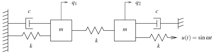
**Figure 5.7:** Coupled spring mass system. Each mass is connected to two springs with stiffness  $k$  and a viscous damper with damping coefficient  $c$ . The mass on the right is drive through a spring connected to a sinusoidally varying attachment.
