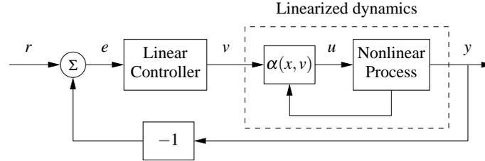
**Figure 5.15:** Feedback linearization using feedback. A nonlinear feedback of the form  $u = \alpha(x, v)$  is used to modify the dynamics of a nonlinear process so that the response from the input  $v$  to the output  $y$  is linear. A linear controller can then be used to regulate the system's dynamics.
