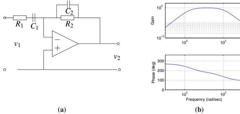
**Figure 5.12:** Active band pass filter. The circuit diagram shows an op amp with two  $RC$  filters arranged to provide a band pass filter. The plot on the right shows the gain and phase of the filter as a function of frequency.
