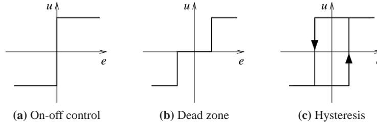
**Figure 1.16:** Input-output characteristics of on-off controllers. Each plot shows the input on the horizontal axis and the corresponding output on the vertical axis. Ideal on-off control is shown in (a), with modifications for a dead zone (b) or hysteresis (c). Note that for on-off control with hysteresis, the output depends on the value of past inputs.
