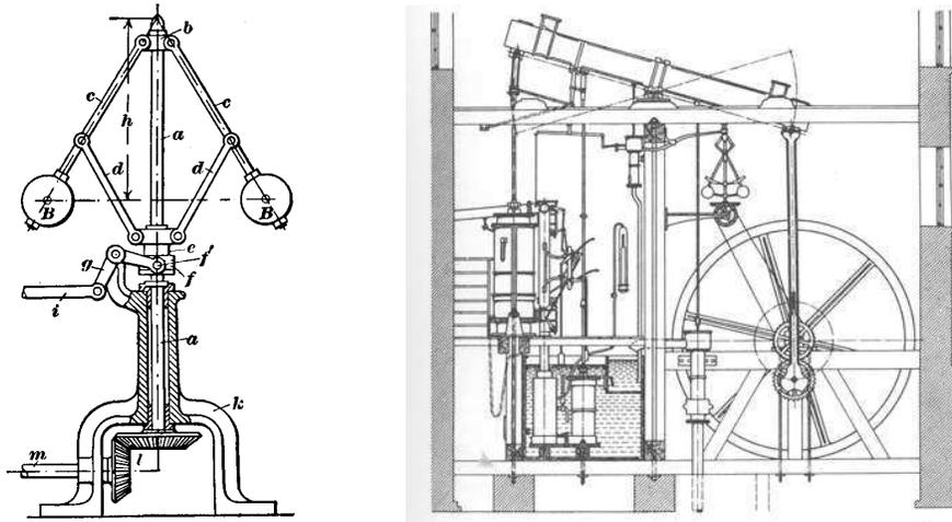
**Figure 1.2:** The centrifugal governor and the Watt steam engine. The centrifugal governor on the left consists of a set of “flyballs” that spread apart as the speed of the engine increases. The Watt engine on the right uses a centrifugal governor (above and to the left of the fly wheel) to regulate its speed. Figures courtesy Richard Adamek (copyright 1999) and Cambridge University.
