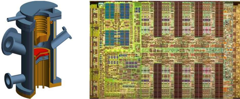
**Figure 1.7:** Materials processing. Modern materials are processed at carefully controlled conditions, using reactors such as the metal organic chemical vapor deposition (MOCVD) reactor shown on the left, which was for manufacturing superconducting thin films. Using lithography, chemical etching, vapor deposition and other techniques, complex devices can be built, such as the IBM cell processor shown on the right. Photographs courtesy of Caltech and IBM.
