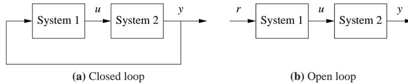
**Figure 1.1:** Open and closed loop systems. (a) The output of system 1 is used as the input of system 2 and the output of system 2 becomes the input of system 1, creating a “closed loop” system. (b) The interconnection between system 2 and system 1 is removed and the system is said to be “open loop”.
