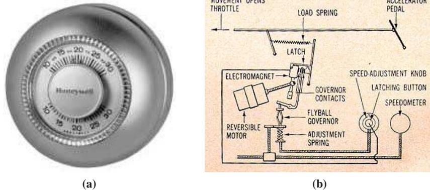
**Figure 1.4:** Early control devices. (a) Honeywell T86 thermostat, originally introduced in 1953. The thermostat controls whether a heater is turned on by comparing the current temperature in a room to a desired value that is set using a dial. (b) Chrysler cruise control system, introduced in the 1958 Chrysler Imperial [Row58]. A centrifugal governor is used to detect the speed of the vehicle and actuate the throttle. The reference speed is specified through an adjustment spring.
