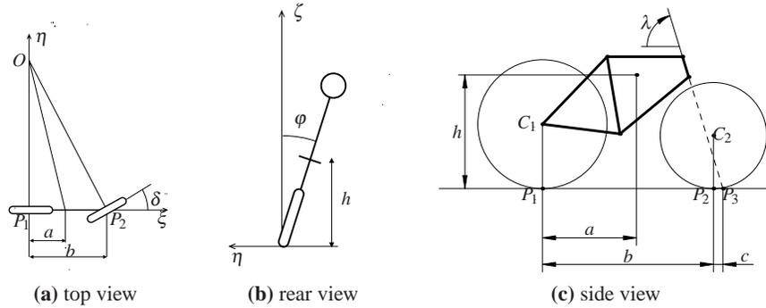
**Figure 3.5:** Schematic views of a bicycle. The steering angle is  $\delta$ , the roll angle is  $\varphi$ . The center of mass has height  $h$  and distance  $a$  from a vertical through the contact point  $P_1$  of the rear wheel. The wheel base is  $b$  and the trail is  $c$ .
