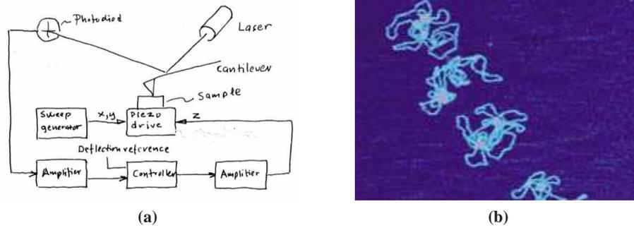
**Figure 3.14:** Atomic force microscope. A schematic diagram of an atomic force microscope is shown on the left, consisting of a piezo drive that scans the sample under the AFM tip. A laser reflects off of the cantilever and is used to measure the deflection of the tip through a feedback controller. An AFM image of DNA is shown on the right.
