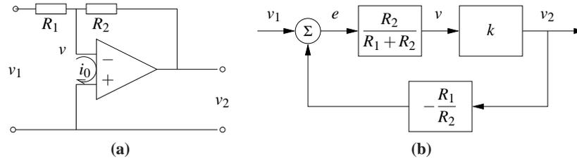
**Figure 3.9:** Stable amplifier using an op amp. The circuit (a) uses negative feedback around an operational amplifier and has a corresponding block diagram (b). The resistors  $R_1$  and  $R_2$  determine the gain of the amplifier.
