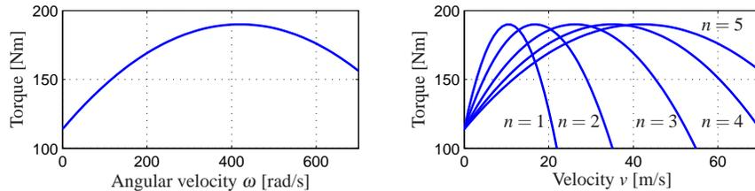
**Figure 3.2:** Torque curves for typical car engine. The graph on the left shows the torque generated by the engine as a function of the angular velocity of the engine, while the curve on the right shows torque as a function of car speed for different gears.
