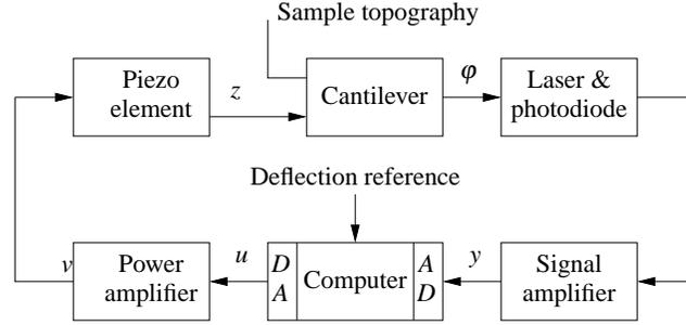
**Figure 3.15:** Block diagram of the system for vertical positioning of the cantilever for an atomic force microscope (AFM) in scanning mode. The control system attempts to keep the cantilever deflection equal to its reference value. Cantilever deflection is measured, amplified and converted to a digital signal, then compared with its reference value. A correcting signal is generated by the computer, converted to analog form, amplified and sent to the piezo element.
