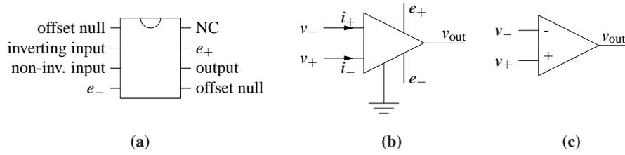
**Figure 3.7:** An operational amplifier and two schematic diagrams. The figure on the left shows the amplifier pin connections on an integrated circuit chip, the middle figure shows a schematic with all connections, and the diagram on the right shows only the signal connections.
