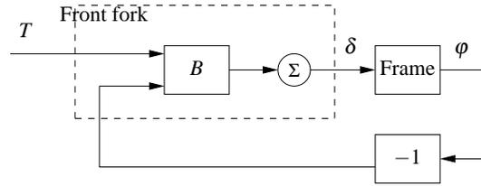
**Figure 3.6:** Block diagram of the bicycle with a front fork. The steering torque applied to the handlebars is  $T$ , the roll angle is  $\phi$ , and the steering angle  $\delta$ . Notice that the front fork creates a feedback from the roll angle  $\phi$  to the steering angle  $\delta$  that under certain conditions can stabilize the system.
