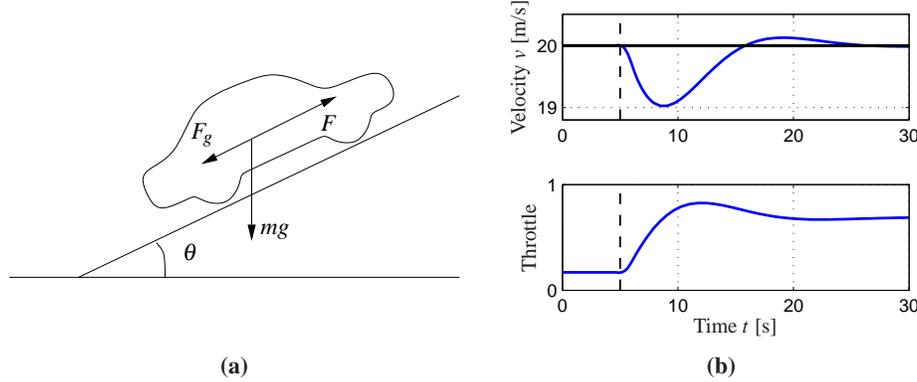
**Figure 3.3:** Car with cruise control encountering a sloping road: a schematic diagram is shown in (a) and (b) shows the response in speed and throttle when a slope of  $4^\circ$  is encountered. The hill is modeled as a net change in hill angle,  $\theta$ , of  $4^\circ$ , with a linear change in the angle between  $t = 5$  and  $t = 6$ . The PI controller has proportional gain is  $k_p = 0.5$  and the integral gain is  $k_i = 0.1$ .
