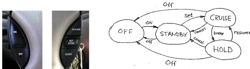
**Figure 3.4:** Finite state machine for cruise control system. The figure on the left shows some typical buttons used to control the system. The controller can be in one of four modes, corresponding to the nodes in the diagram on the right. Transition between the modes is controlled by pressing one of five buttons on the cruise control interface: on, off, set/accel, resume or cancel.
