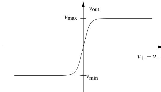
**Figure 3.8:** Input/output characteristics of an operational amplifier. The differential input is given by  $v_+ - v_-$ . The output voltage is a linear function of the input in a small range around 0, with saturation at  $v_{\min}$  and  $v_{\max}$ . In the linear regime the op amp has high gain.
