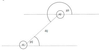
Fig. 3. Basic concept behind localization error detection Fig. 3 shows that nodes  $n_i$  and  $n_j$  see each other with the angles  $P_{ij}$ ,  $P_{ji}$ . These two nodes have a distance of  $d_{ij}$  from each other. Then coordination of  $n_j$  to ni is obtained from:
