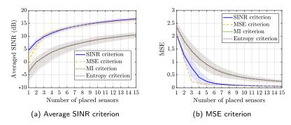
Figure 3: The performances of the SINR and MSE criteria in sensor placement for source separation are compared with the classical sensor placement criteria. Two measures are used to assess the quality of source separation: (a) Average of the SINRs of the separated sources. (b) MSE of the source separation. The curves (resp. shadows) represent the average value (resp. standard deviation around the mean) obtained from Monte Carlo simulations.
