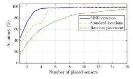
Figure 12: BCI accuracy obtained from electrodes configured using three placement approaches, averaged over 40 subjects
