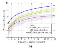
Figure 9: Comparing the sequential approach, where perfect or BSS estimation of the spatial gains is performed in each step, with the greedy method, where the knowledge about the spatial gains remains constant across steps. Two cases are considered: (a) Low level of uncertainty with  $\sigma_u = 0.3$ , and (b) High level of uncertainty with  $\sigma_u = 0.8$ .
