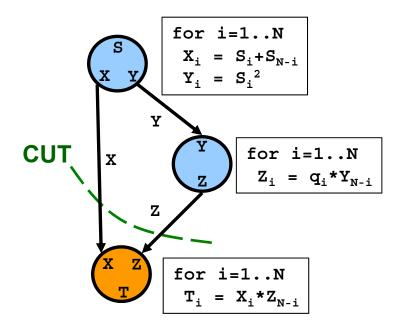
1 / Throughput =  $W_{G1}$   $C_{CUT}$   $C_{CUT}$   $W_{G2}$ Exec. Period= Max{  $W_1+W_2+N+N$  ,  $N+N+W_3$  }
