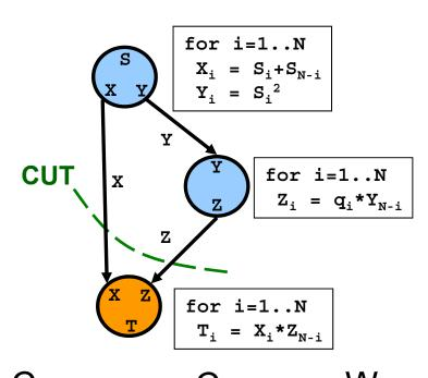
$W_{G1}$   $C_{CUT}$   $C_{CUT}$   $W_{G2}$  Exec. Period= Max{ $W_1+W_2+OV+N+N$ , hop,  $N+N+OV+W_3$ }
