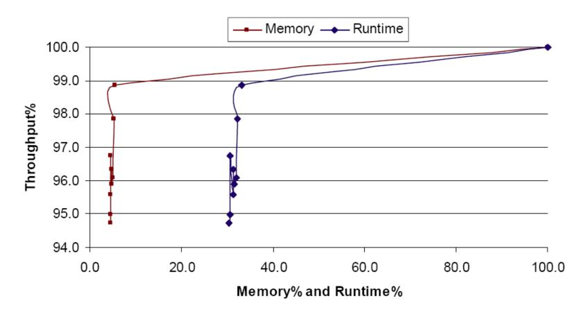
Throughput degradation versus reduction in runtime and memory consumptions when using the approximate partitioning algorithm. All values are normalized against the exact algorithm.
