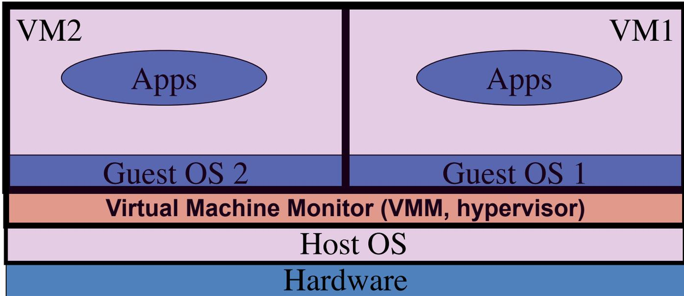
single HW platform with isolated components
