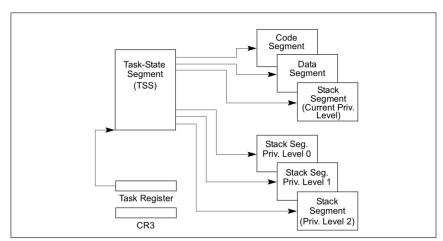
Figure 7-1. Structure of a Task
