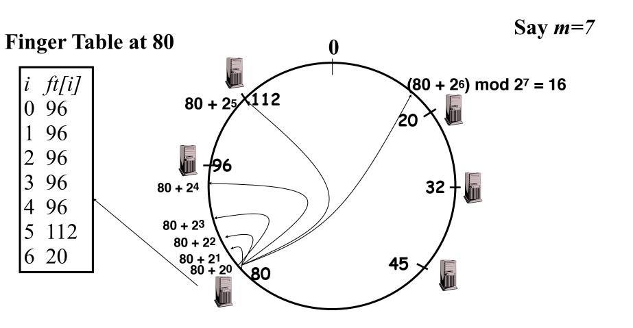
*i*th entry at peer with id *n* is first peer with id  $\geq n + 2^i \pmod{2^m}$
