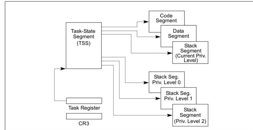
Figure 7-1. Structure of a Task
