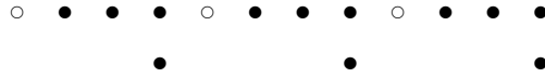
Fig. 6.10. A canonical WBS encoding of an extended hybrid-redundant number system with digit set [-8, 8]
