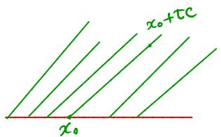
$$\left\{ \begin{array}{l} u_t + c u_x = 0 \\ u(x, 0) = \sin x \quad 0 < x < \pi \end{array} \right.$$
