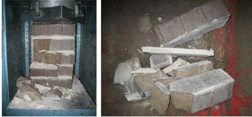
Fig. 10. The damaged specimen after compression test.
