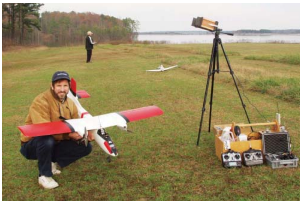
MICRO DRONE: Adding a video camera and radio downlink to a radio-controlled model airplane has become easy.
