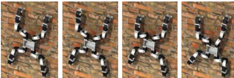
ANIMAL WRIGHT: Israeli robot researcher Amir Shapiro [top] builds snakelike robots (like the one draped around his neck) that can twist like screws. He also makes robots that scale walls [bottom] by releasing tiny amounts of glue, much as a snail leaves a trail of MUCUS. PHOTOS: TOP, DANI MACHLIS/BEN-GURION UNIVERSITY; BOTTOM, TOMER AVRAMOVITCH AND AVISHAI SINTOV
