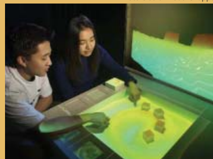
The SandScape allows users to design landscape manipulating sand-based topography and simulating shadow, water drainage, and other aspects.
