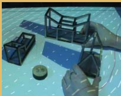
The Urban Planning Simulation ("Urp") allows users to manipulate physical building models to explore shadow and wind flow.
