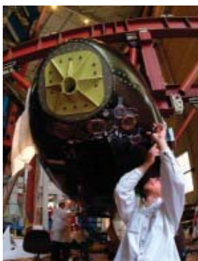
RESKINNED BIRD: A technician adjusts panels on an early version of the X-37B.
