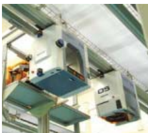
CHIP TRIP: Materials-handling equipment used in semiconductor manufacturing is often powered inductively.
