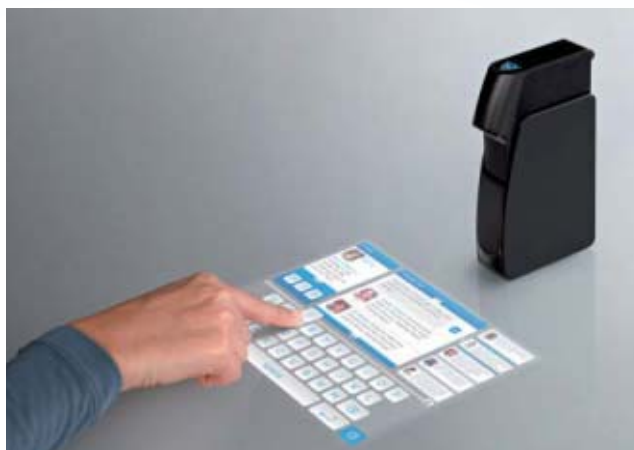
LIGHT TOUCH: This projection system creates a picture from holograms, then uses lasers [above] to project an interactive image onto a tabletop [left].
