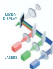
LIGHT TOUCH: This projection system creates a picture from holograms, then uses lasers [above] to project an interactive image onto a tabletop [left].
