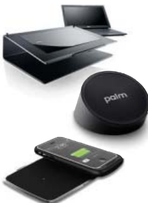
NO-CORD CHARGING: Wireless charging pads are becoming widely available for consumer electronics, including the Dell Latitude Z laptop [top], the Palm Pre smartphone [center], and various smartphones equipped with Powermat charging sleeves [bottom].
