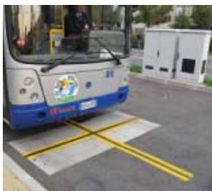
WIRELESS CHARGING: Electric buses in the ancient port area of Genoa, Italy, are recharged inductively.
