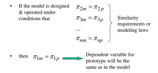
Flow conditions for a model test are completely similar if all relevant dimensionless parameters have the same corresponding values for the model and the prototype.
