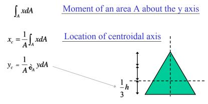
For a plate of uniform thickness the intersection of the centroidal axes is also the center of gravity
