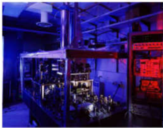
NIST-F1 time and frequency standards: 1 sec = 9,191,631,770 period of the resonance frequency of a Cs-133 atom
