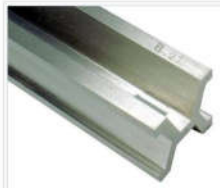
Closeup of National Prototype Metre Bar No. 27, made in 1889 by the International Bureau of Weights and Measures (BIPM) and given to the United States, which served as the standard for defining all units of length in the US from 1893 to 1960
