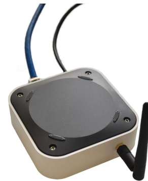
Fig. 2. The IIoT-based thermostat for controlling split air conditioners.
