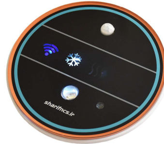
Fig. 2. The IIoT-based thermostat for controlling split air conditioners.
