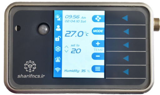
Fig. 1. The IIoT-based thermostat for controlling FCUs.
