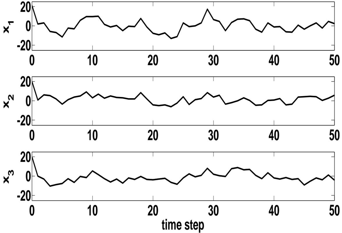
Fig. 7. State trajectories of the controlled system of [12] when variances of channel noise in exchanging measurements and controls are 0.1 and 10, respectively, and attenuation factors are 1.
