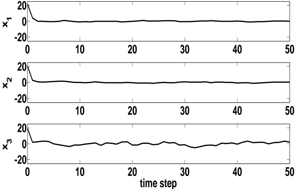
Fig. 4. State trajectories of the controlled system when variances of channel noise in exchanging measurements and controls are 0.1 and 1, respectively, and attenuation factors are 1.
