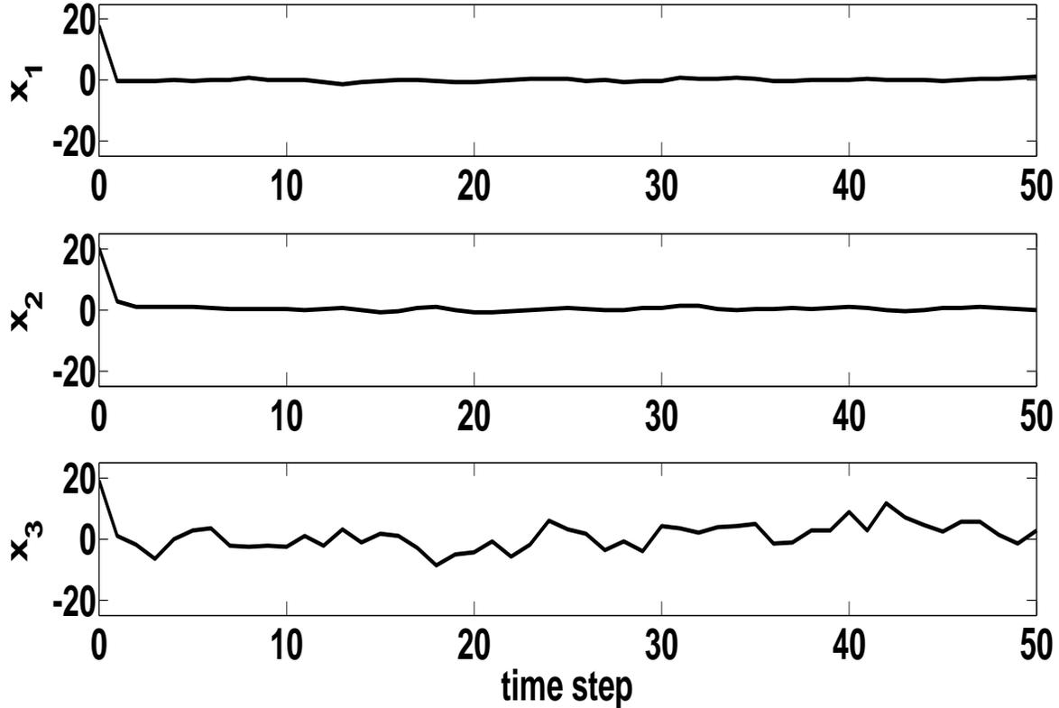
Fig. 6. State trajectories of the controlled system when variances of channel noise in exchanging measurements and controls are 0.1 and 10, respectively, and attenuation factors are 1.
