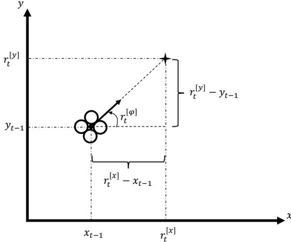
Fig. 4. An autonomous vehicle with positions  $x_{t-1}$  and  $y_{t-1}$  moving towards the desired positions  $r_t^{[x]}$  and  $r_t^{[y]}$ .
