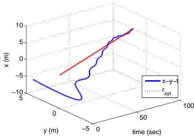
Fig. 12.  $x_t - y_t - time$  diagram for  $\alpha = 0.9$  when the feedback linearization technique of [19] is applied.
