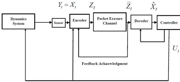
Fig. 1. A dynamics system controlled over the packet erasure channel with feedback acknowledgment.
