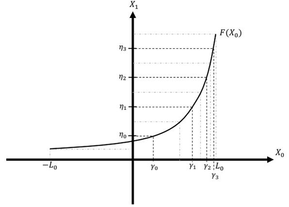
Fig. 2. Equal sized, non-overlapping sub-intervals for encoding with  $R = 2$ .
