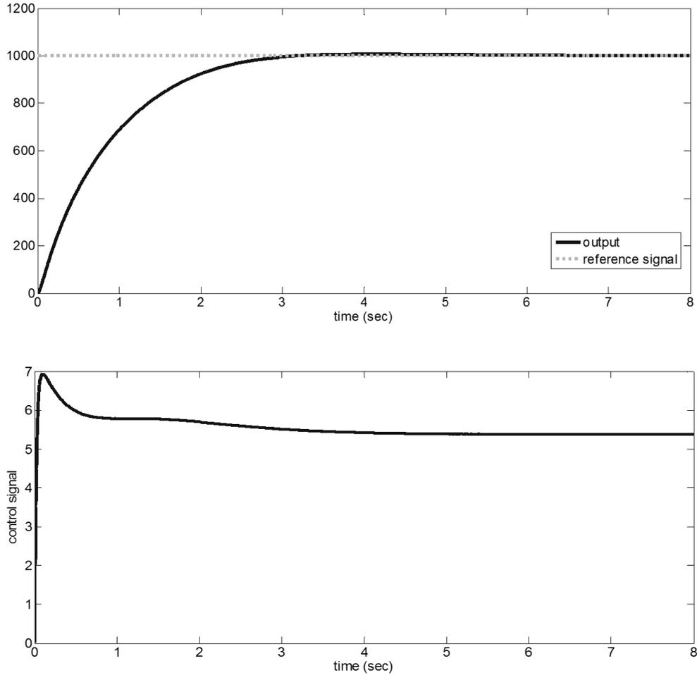
Fig. 5. The response of the system and control signal for  $r(t) = 1000 \text{ rad/s}$ .
