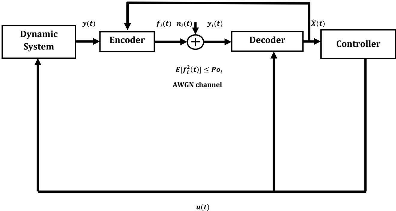
Fig. 1. A dynamic system over MIMO AWGN channel.
