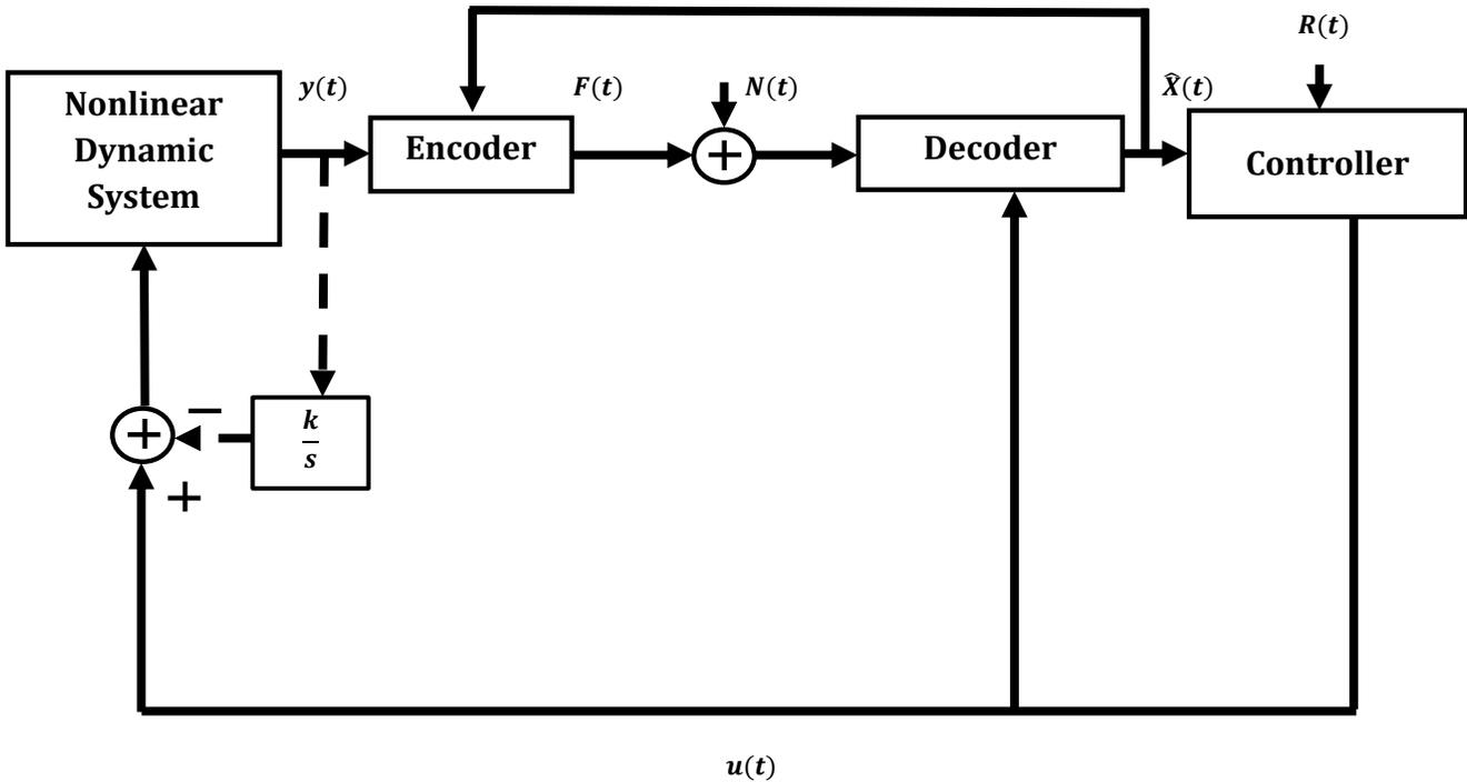
Fig. 2. Nonlinear dynamic system (1) controlled over AWGN channel.
