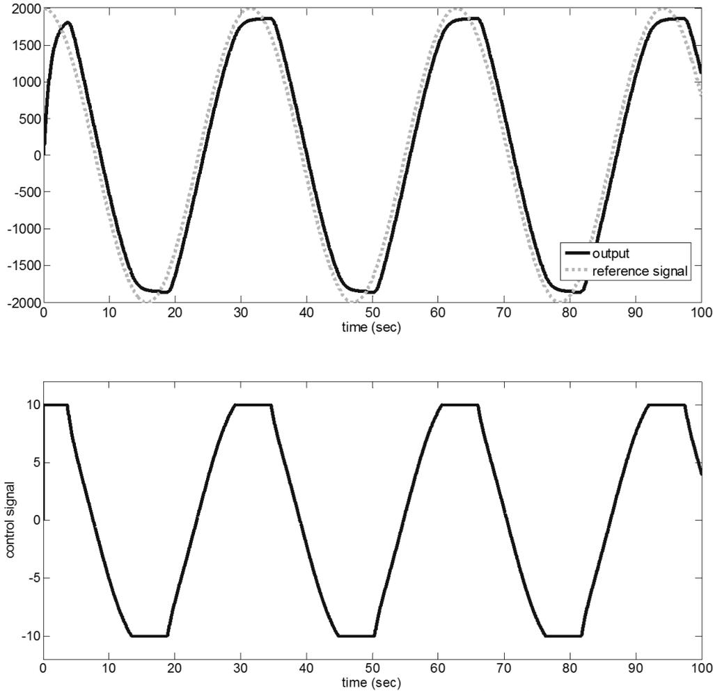
Fig. 7. The response of the system and control signal for  $r(t) = 2000 \cos(0.2t)$  rad/s.
