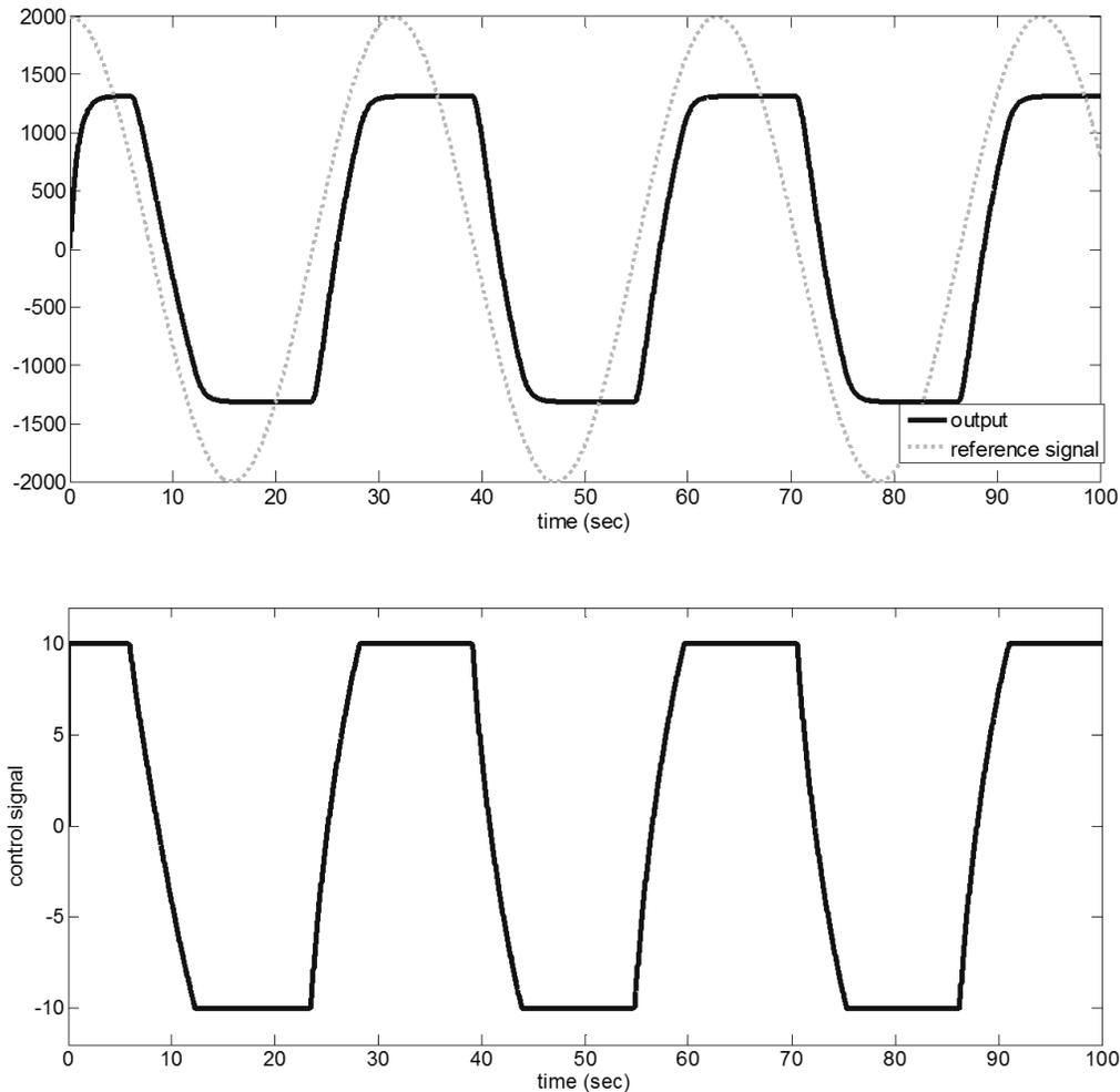
Fig. 8. The response of the system and control signal of the linear method of [10] for  $r(t) = 2000 \cos(0.2t)$  rad/s.
