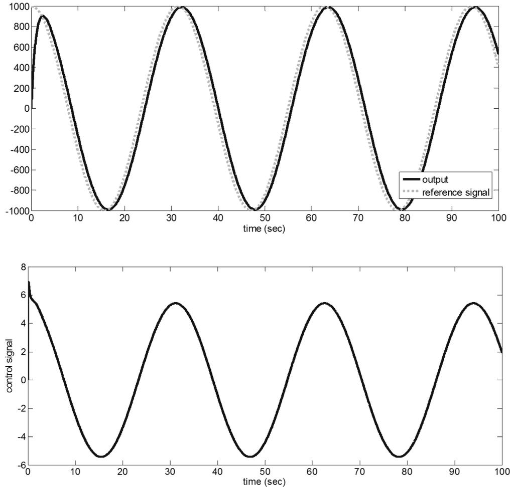
Fig. 6. The response of the system and control signal for  $r(t) = 1000 \cos(0.2t) \text{ rad/s}$ .
