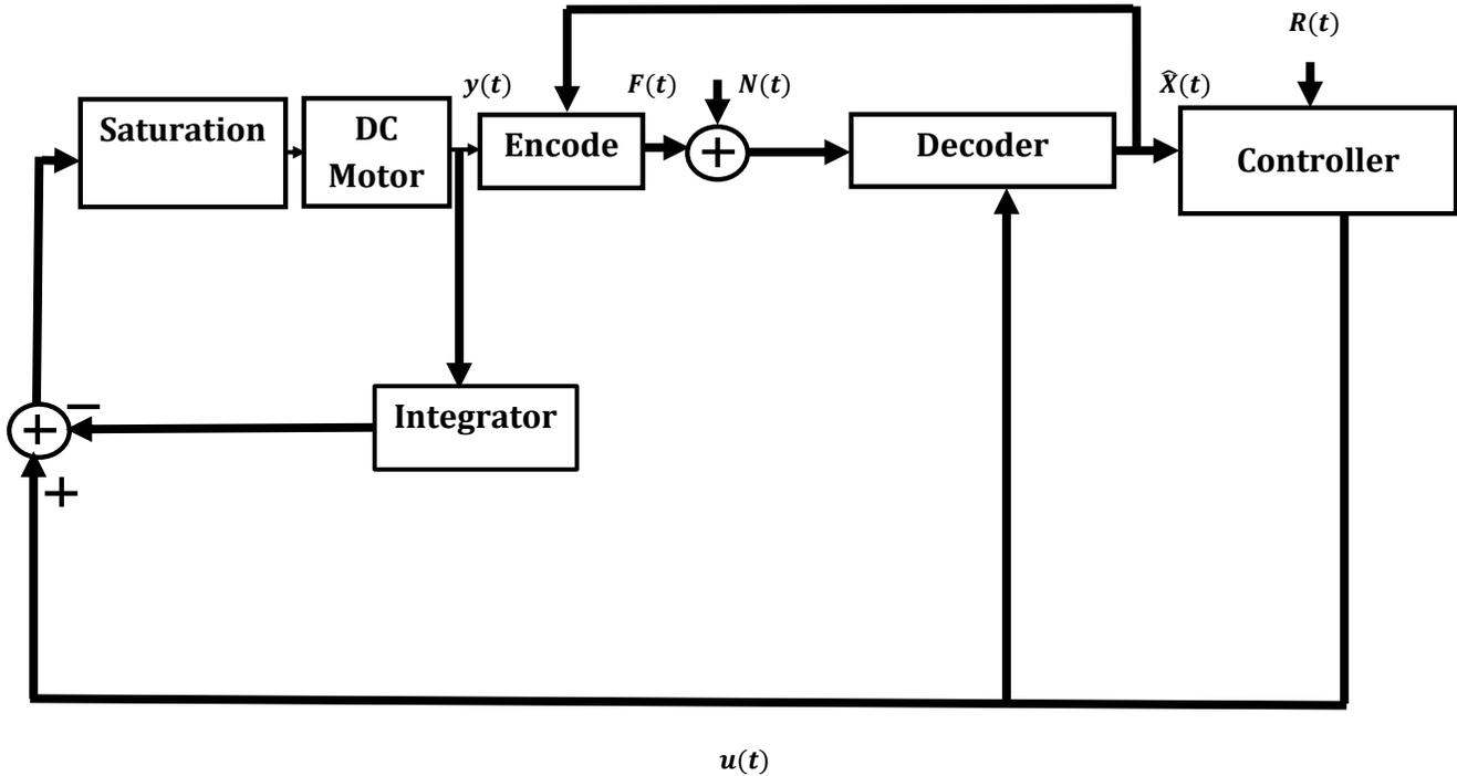
Fig. 3. A nonlinear dynamic system controlled over AWGN channel.
