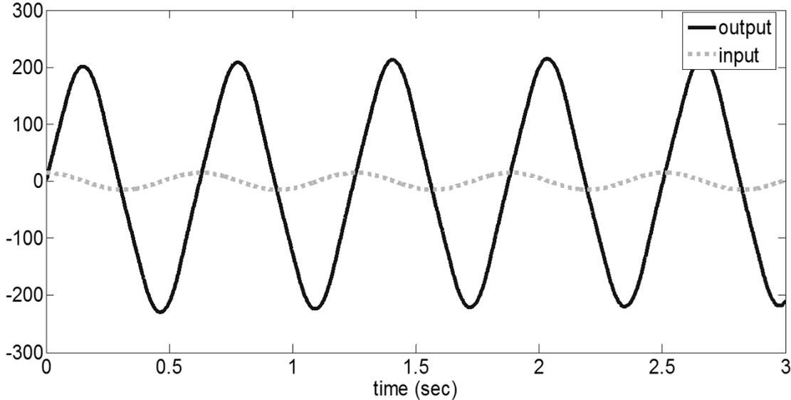
Fig. 4. The output of the nonlinear system for the sinusoidal input  $u(t) = 15 \cos(10t)$  and  $x(0) = 1$ .
