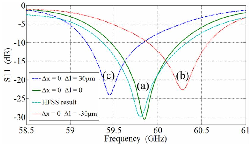
Fig.1: S11 for three cases where slot offsets remained equal to original design values
