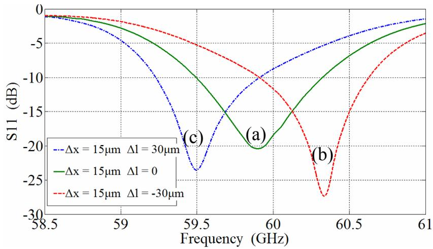
Fig.3: S11 for three different slot lengths. Slot offsets increased from their nominal value
