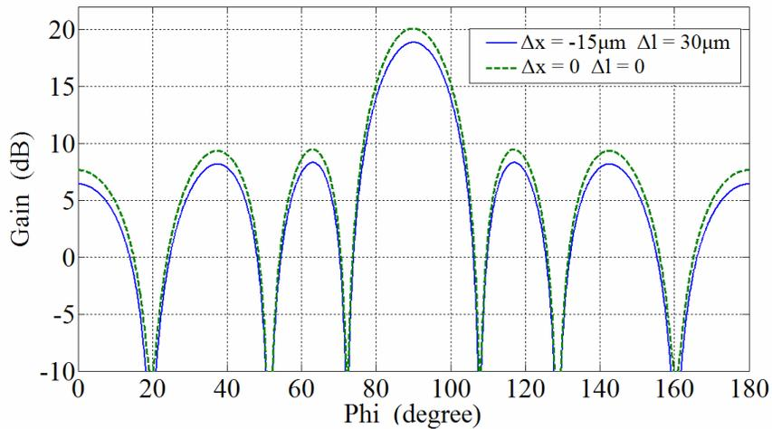
Fig.4: Gain of the original array and that of the worst case array at 60GHz
