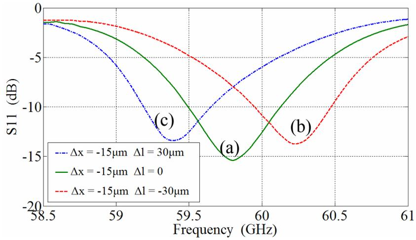
Fig.2: S11 for three different slot lengths. Slot offsets reduced from their nominal values
